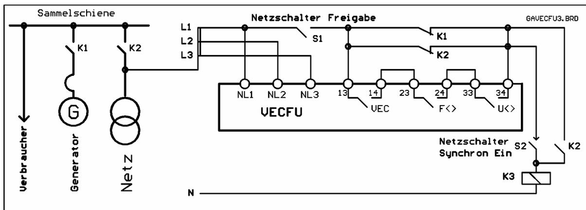
**Note:** Only one phase (L1 in this case) is necessary for detecting and measuring the phase change of the protective unit VECFU3 as the phase changes of the phase L1 also take place in all other phases with the same phase changes (frequency and phase are interconnected in three-conductor power supplies).
