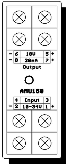
The Measuring Transducer AMU is used to transform an AC current to an 0/4-20mA or 0/2-10V output signal for driving display units and controls. The potential separation of the measuring circuit from the output circuit and the supply voltage (10-34VDC) make the AMU150/110 suitable in particular for use in disturbed environments and with ambiguous potentials. This allows the unit to also measure AC currents on other voltage levels.
