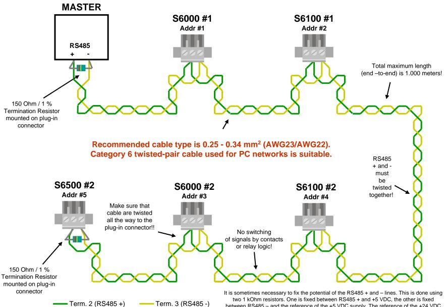
two 1 kOhm resistors. One is fixed between RS485 + and +5 VDC, the other is fixed between RS485 - and the reference of the +5 VDC supply. The reference of the +24 VDC supply must then be connected to terminal 1 of the RS485 plug on each and every SIGMA module.
