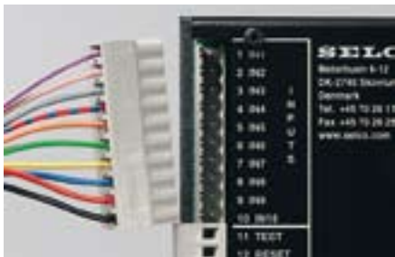
Figure 4: Rear Side Input Terminals.
