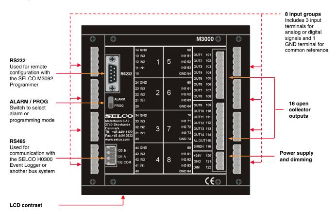
The M3000 includes 8 groups of input terminals. Each group is physically represented by a plug-in connector that holds 3 input terminals, "IN1", "IN2" and "IN3", and one common reference terminal "GND". Be sure not to confuse the physical inputs with the logical inputs "INA", "INB" and "INC". The logical inputs has no related input terminals, they are imaginary inputs intended for average calculation based upon other inputs. The logical inputs are described later in this manual.
