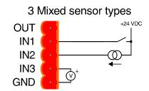
The example above shows 3 different sensors connected to the same input plug-in connector. Input terminal "IN1" is connected to a potential free contact to +24V DC.
