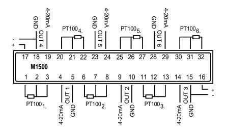
The example below shows connections to one input group of M3000. For more details see separate data sheet M1595.
