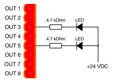
The open collector output "AL.OUT" can be used to signal the appearance of multiple alarms controlling the same output.
