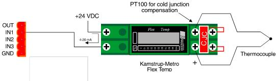
The transmitter snown above works like a current gate. It releases only 4mA at 0°C and 20mA at 100°C.
