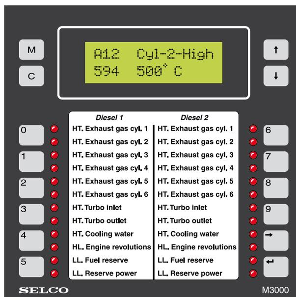
indicate new alarms with flashing light and acknowledged (reset) alarms with steady light. The user can acknowledge all new alarms by pressing the "C" key.
