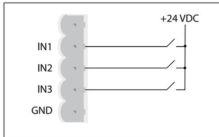
Fig. 3. 3 x Contact inputs.
