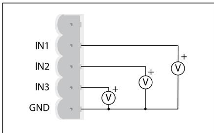
Fig. 1. 3 x Voltage inputs.
