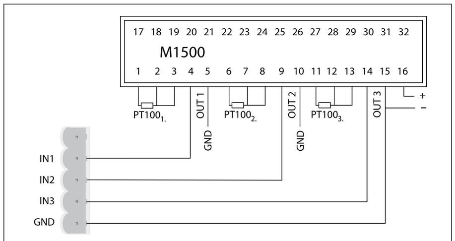
Fig. 5. 3 x PT100 transmitters.
