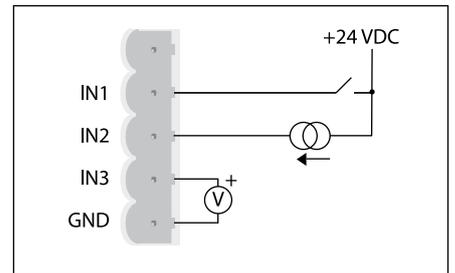
Fig. 4. 3 x Mixed sensor types.
