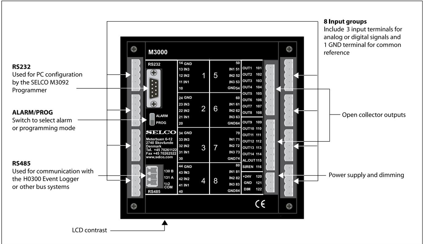
The input plug-in connectors will later on be referred to as "input groups". Each input can be configured for current or voltage input. Fig. 1 to 5 illustrate possible input group configurations which can be arranged as follows:
