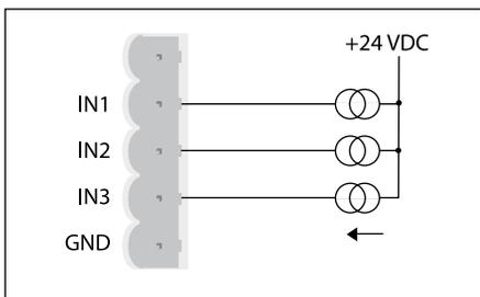
Fig. 2. 3 x Current inputs.
